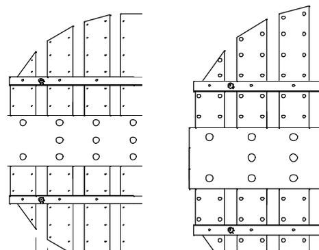
Proper installation of the liquid distribution system is essential to achieve the design standard of liquid distribution quality and good overall operation of the packed bed. The distribution troughs and parting box must be leveled to within  $\pm 4\text{mm}$  in accordance with the installation instructions supplied with the TD Liquid Distributors.
