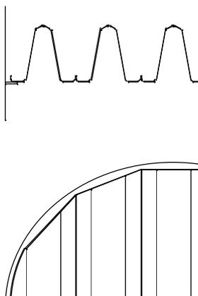
The AlphaPLUS™ PSG070 is a flat bar type support grid designed for use with structured packing. The standard grid is made up in 375mm wide segmental sections which can be installed through column manways (minimum manway size 450mm NB) and bolted together inside the column. The standard design has grid bars spaced on 75mm centres but variations with closer grid spacings can be manufactured to support random packings where the support plate capacity is not critical.
