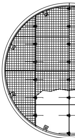
The AlphaPLUS™ DSP300 is designed to function both as a support plate for random packing and as a collector/distributor/support plate for the dispersed phase in liquid-liquid extraction columns.
