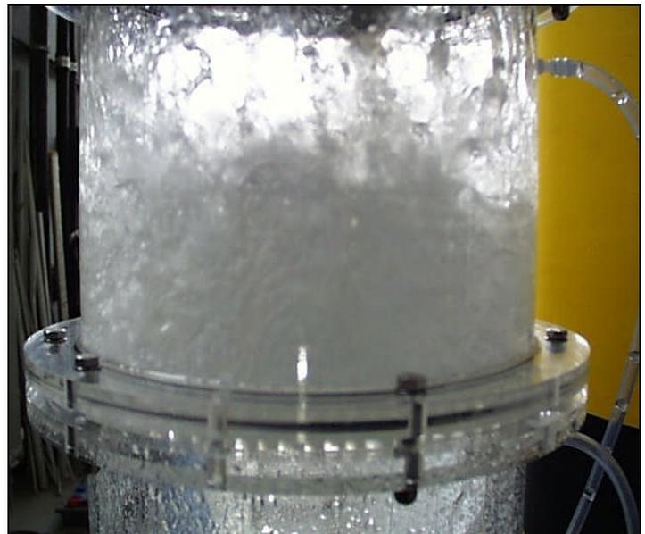
Fig.4: View of the Tray During Operation
